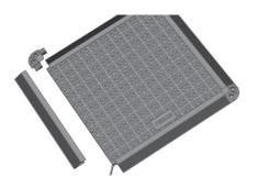
2. Install the aluminum alloy blank and the corner connecting the aluminum alloy blank
